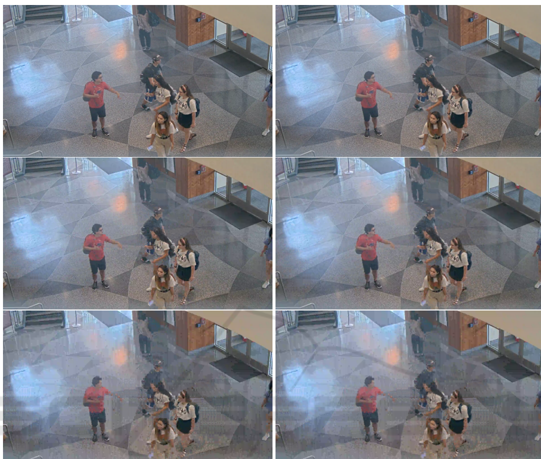
Figure 1: Example frame of video compressed using different compression parameters and corresponding distorted images. Left column shows the images compressed with compression parameters CRF-35, CRF-41, CRF-47 respectively. Right columns show the corresponding blurred image.
