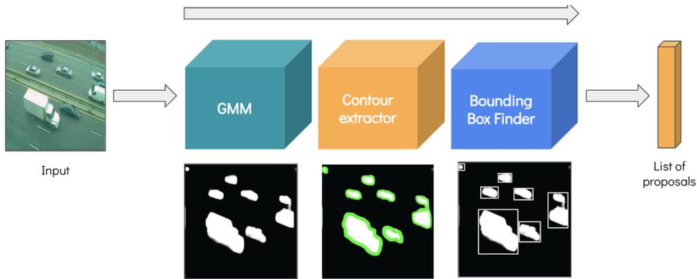
Figure 2: Gaussian-based Region Proposal Model.
