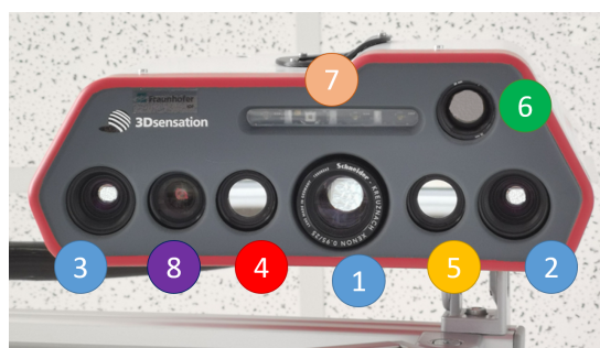
Figure 1: Sensor head composed of a GOBO projector (1), two NIR cameras at 850 nm (2, 3), a NIR camera at 780 nm (4), a NIR camera at 940 nm (5), a thermal camera (6), an LED array with LEDs at 780 nm and 940 nm (7), and a reserved color camera (8).
