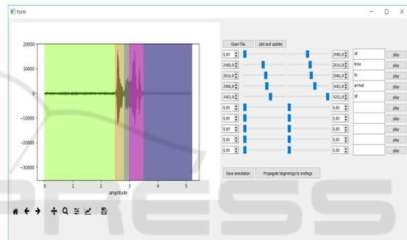
Figure 5: The developed GUI to check the automated annotation. If the automated annotation fails for some reason, the GUI allows for modifying both text labels and speech intervals.
