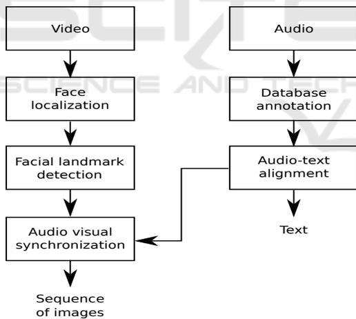
Figure 3: Database generation pipeline.
