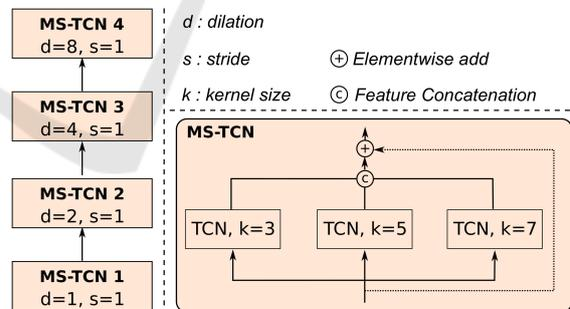
Figure 2: Sequence back-end network: it contains four layers of Multi-scale dilated TCN, where the dilation size of each layer is 1, 2, 4, and 8, respectively. Each layer consists of three TCN blocks with kernel sizes 3, 5, and 7, respectively.
