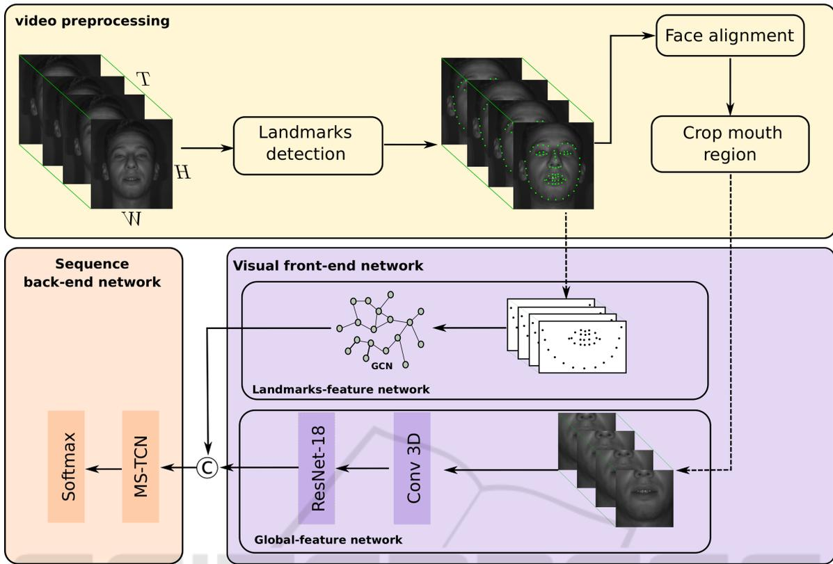
Figure 1: Three stages framework of the proposed system. Video preprocessing: extract facial landmarks and crop the mouth region from the input infrared video. Visual front-end network: encode global visual and lips contour variation on the cropped mouth area. Sequence back-end network: based on a multi-scale temporal convolutional network (MS-TCN) to encode temporal variation along the extracted features and classify the input video.
