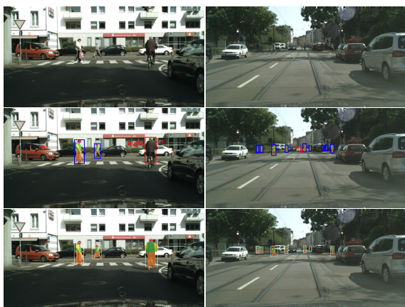
Figure 2: Inference results: original image (top row), ground truth bounding boxes in blue, ignored bounding boxes in red and ground truth body part segmentation (middle row) and ConDA predictions (bottom row).
