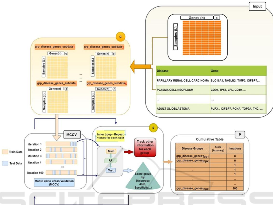
Figure 1: Illustration of the GediNETPro. The input panel contains the gene expression data and the grouping table. Component G creates the sub\_datasets based on the Input panel. The MCCV panel uses the S component to perform the looping. The P component tracks the output of MCCV and S to be stored as a cumulative table.
