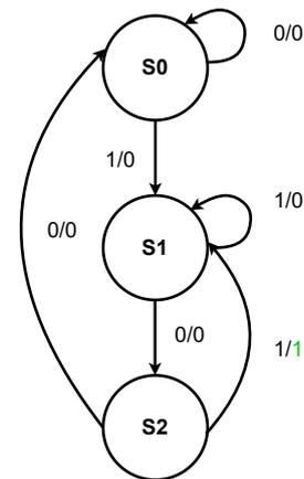
Figure 1: FSM of 3-bit '101' SD.
