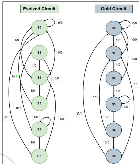
Figure 6: Comparison of gold vs evolved FSM of 6-bit '111000' SD.
