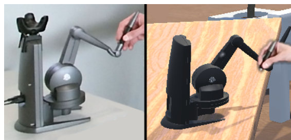
Figure 13: Left: The 3D Systems Touch X with an HTC VIVE Tracker (3.0). Right: The virtual device tracked in the VE.
