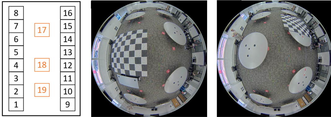
(a) Layout of chessboard mats (b) Chessboard mat at position #4 (c) Chessboard mat at position #13 Figure 3: Illustration of chessboard-mat layout used for training the MLP model.
