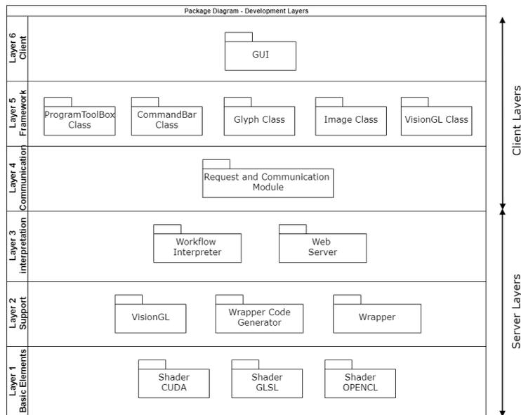
Figure 1: Package diagram: development layers (Maciel et al., 2021).
