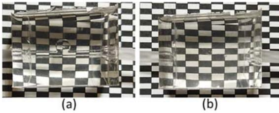
Figure 2: Evaluation of the optical transparency of the biomodel with the fluid: (a) water and (b) glycerin-based solution.
