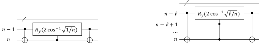
Figure 1: B_{n,1} gate (left) and B_{n,\ell} gate for 2 \leq \ell \leq k (right).
