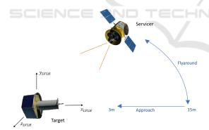
Figure 10: Schematic representation of the rendezvous trajectory.
