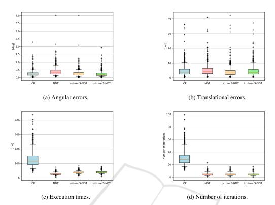
Figure 5: Distribution of the errors and key characteristics of each algorithm, when performing pairwise scan registration from scan 22 to 923 of the *Hanover 2* dataset.
