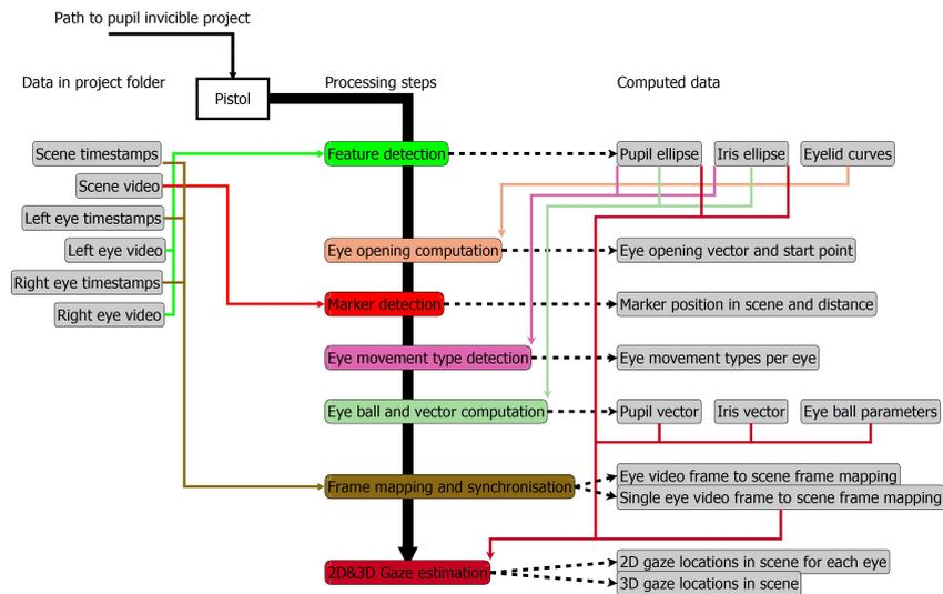
Figure 1: The workflow of Pistol. In gray are the data sources, and the single processing steps are in color. Each arrow corresponding to a data dependency is colored in the same color as the processing step.
