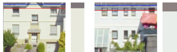
Figure 12: The blue lines separate the roof and facade based on an edge image, the red lines separate the dominant colors of the roof and facade.
