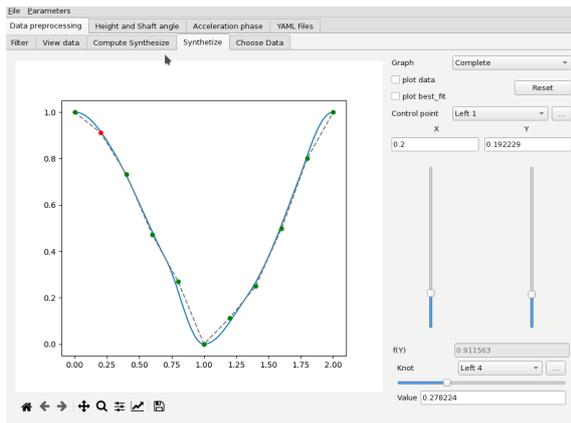
Figure 7: SPRing input GUI showing the synthesis of a given sweep angle with B-spline.
