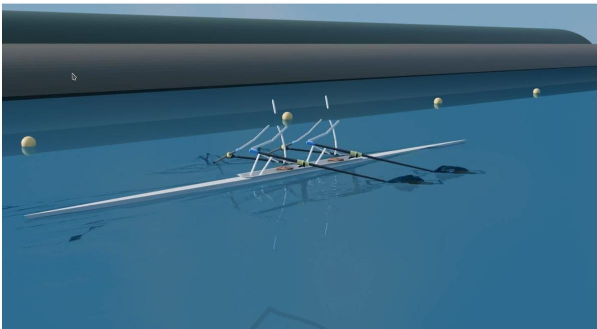
Figure 9: Stickman rendering of a double scull with a co-simulation SPRing/ISIS-CFD. Morphology and gesture signature can be defined specifically for each rower.
