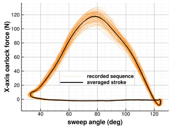
Figure 2: Force as a function of sweep angle, raw data and averaged procedure.
