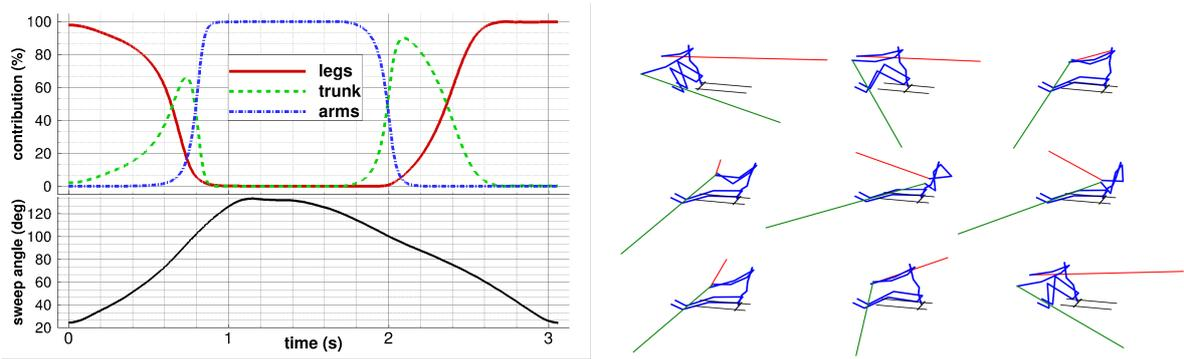
Figure 5: On the top left, contribution of legs bending, trunk inclination and arms bending to the oar rotation as a function of time, resulting on the incremental procedure. On the bottom left, averaged sweep angle as a function of time coming from measurement. On the right, resulting sequence of rower postures for a whole rowing stroke.
