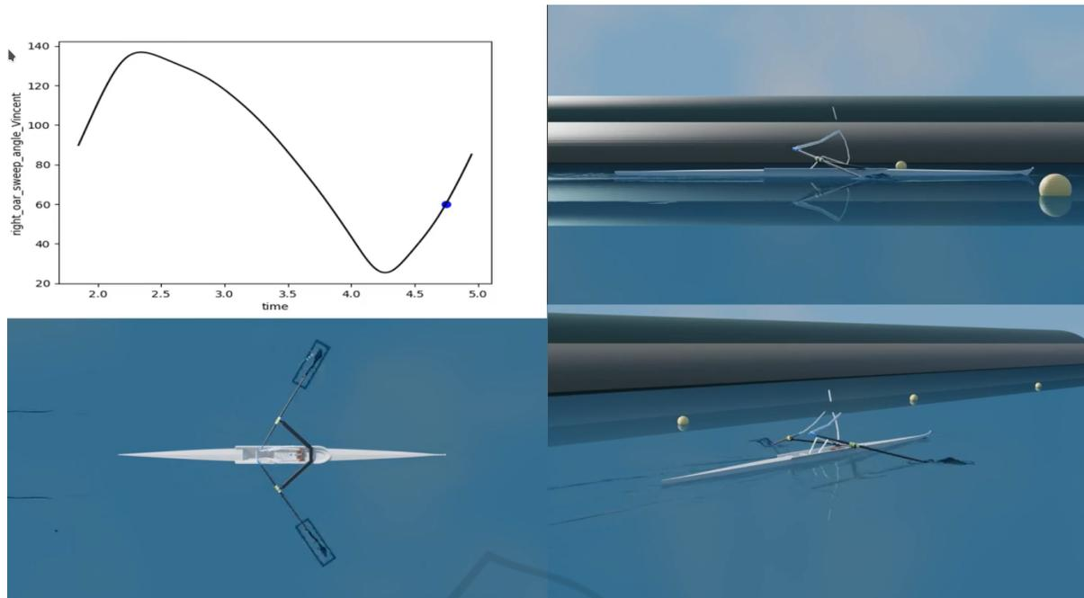
Figure 10: Multi-view stickman rendering, synchronized with the graph showing the sweep angle as a function of time, made by the SPRing output GUI.
