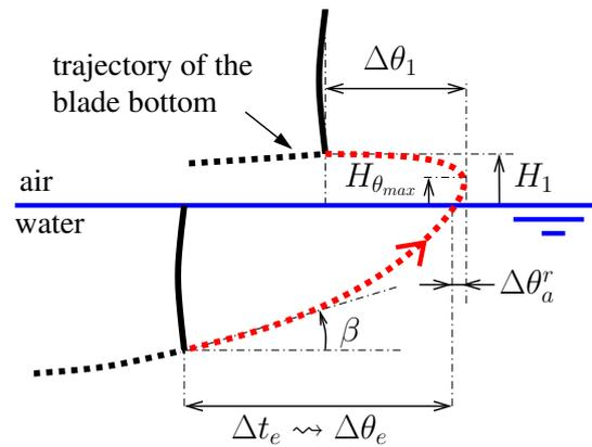
Figure 4: Parametrization of the vertical motion of the blade during the release phase.
