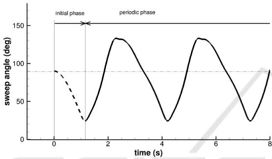
Figure 6: Imposed sweep angle as a function of time including the initial phase.
