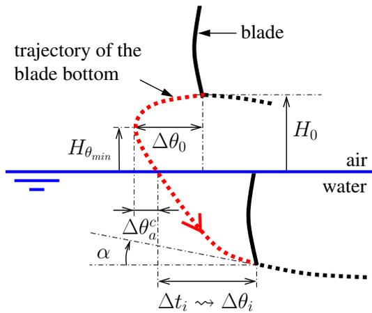
Figure 3: Parametrization of the vertical motion of the blade during the catch phase.
