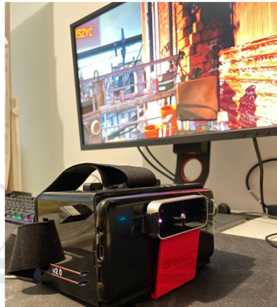
Figure 6: DreamzVR 2.0 goggles with an installed smartphone and a front-mounted Leap Motion camera running Half-Life: Alyx.
