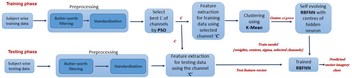
Figure 2: Flow diagram of proposed model.
