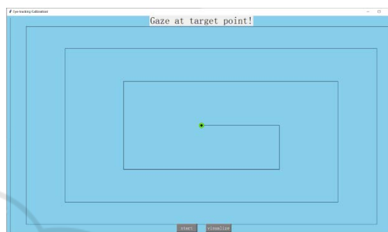
Figure 2: Spatially nonuniform square spiral trace on the X-Y plane with limited speed designed for model learning.
