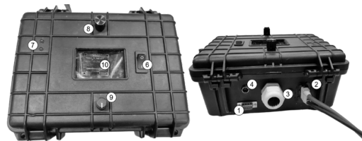
Figure 9: Housing for the electronic components (Doblaski, 2021).
