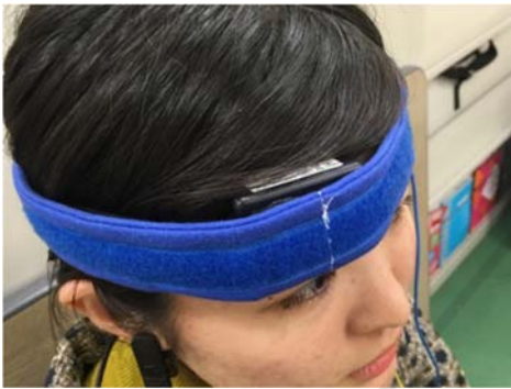
Figure 2: The HEG sensor and its installation.
