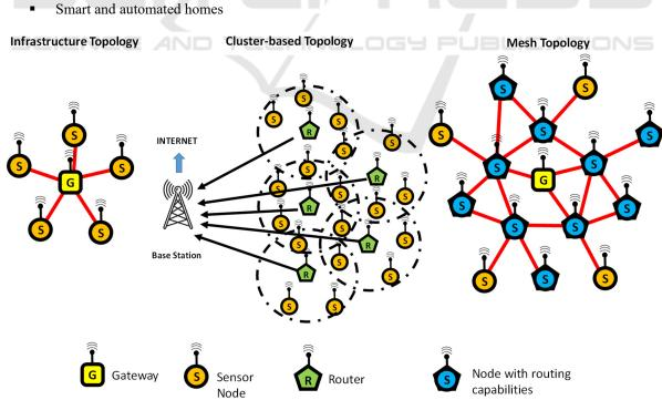
Figure 1: Topologies used in WSNs.
