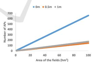
Figure 9: Number of APs per area of the field for the emitter at 2 m.
