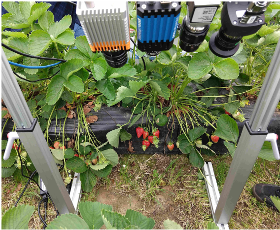
Figure 7: Setup used for a first in-field data collection. A rigid frame carries four cameras used to collect the multi-spectral data. In this setting the frame is placed between the ridges.
