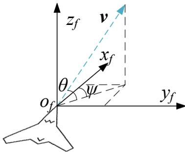
Figure 1: Inertial Coordinate System.
