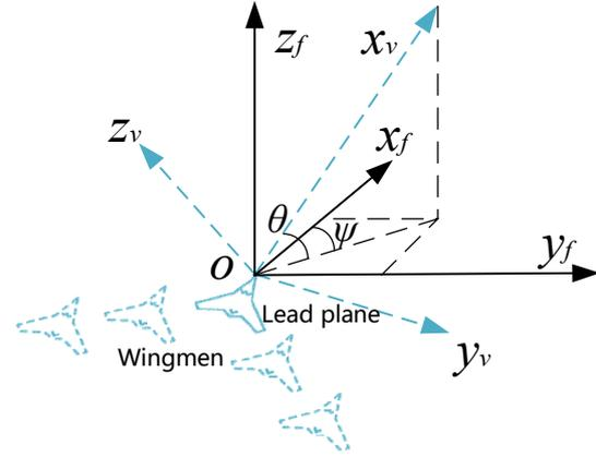
Figure 3: Method for Determining Wingmen Target Point.
