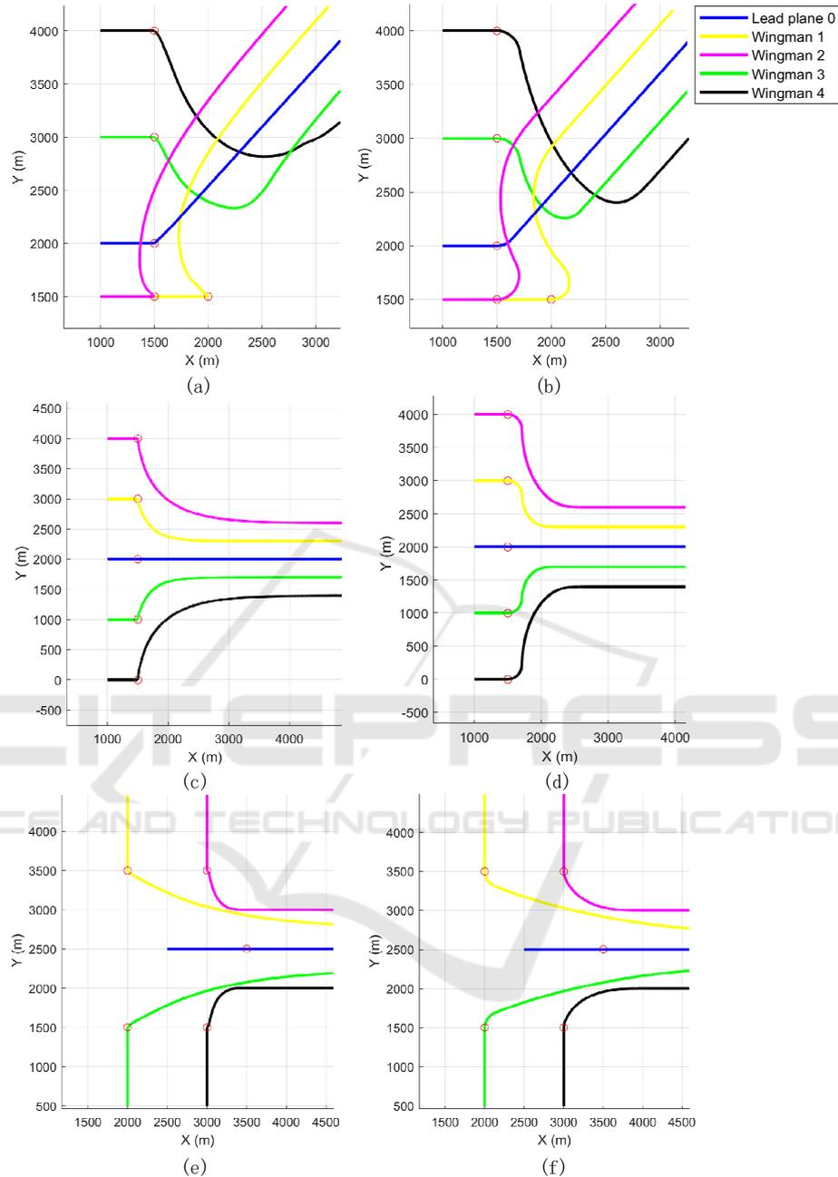
Figure 5: Trajectories generated based on the traditional model and the model proposed in this paper. (a, c, and e): traditional model; (b, d, and f): model proposed in this paper).
