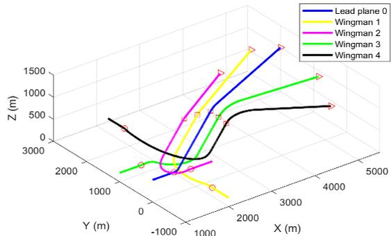
Figure 7: Formation flying and decentralization trajectory planning of UAVs.
