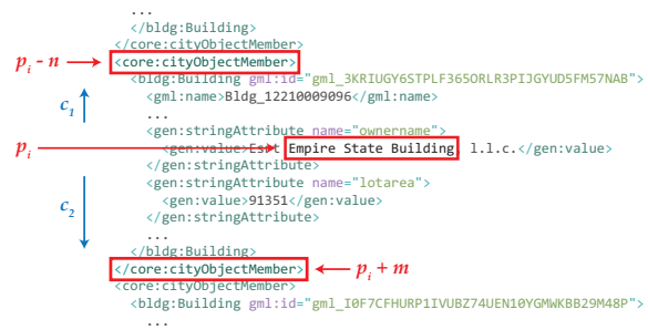
Figure 1: General approach to search in a text file and extract a CityGML building containing the match at position p_i and ranging from p_i - n to p_i + m
