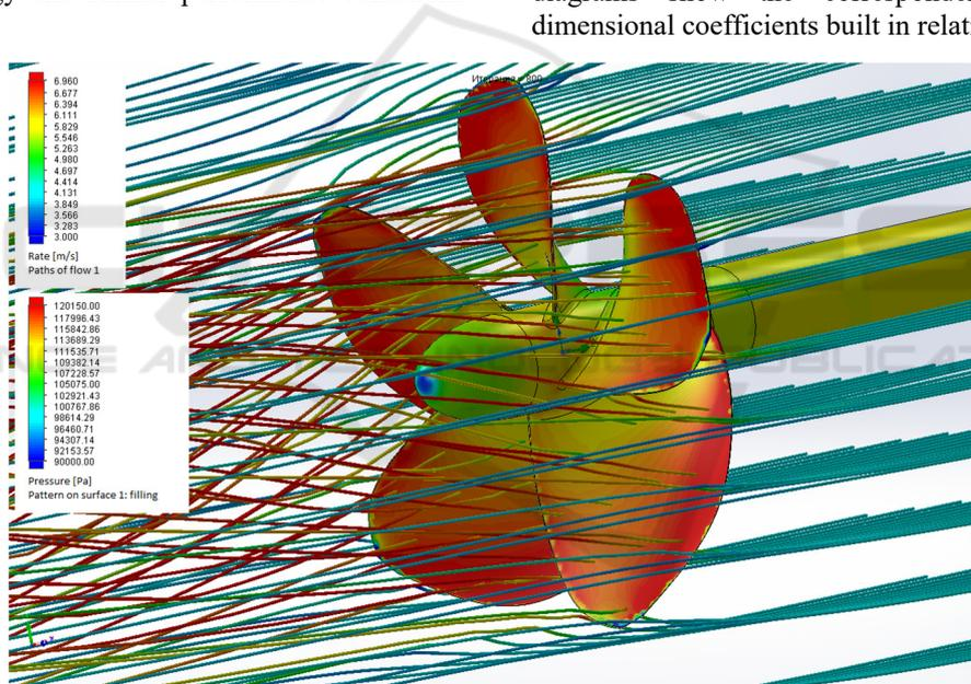
Figure 1: Propeller B 5.105.1.4 (the visualization pattern of computer simulation:  $v=4$  m/sec,  $n=500$  rpm).
