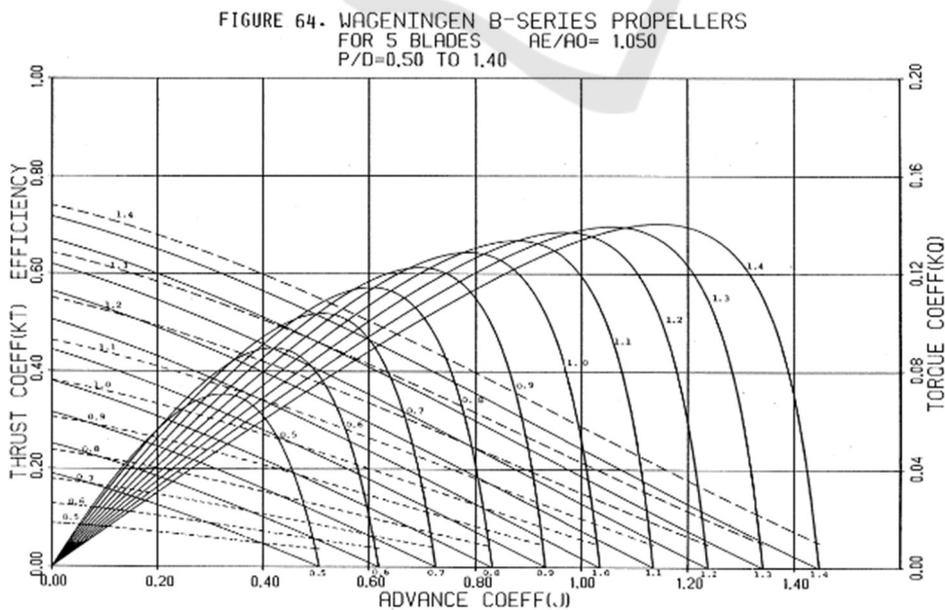
Figure 2: Performance curves of the propeller.
