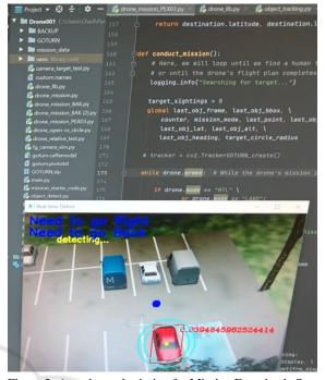
Figure 3: A student submission for Mission Exercise 1. Students must demonstrate that their code (top) can safely operate the drone in the SITL environment (bottom) before being run on real-world hardware.
