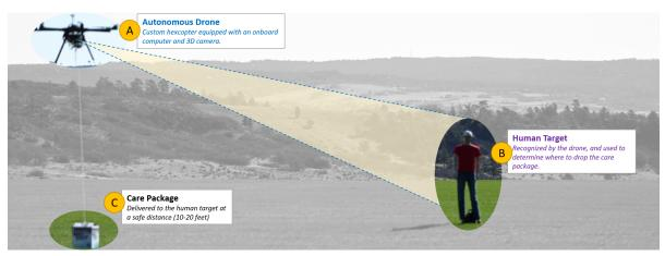
Figure 1: A summary of CS 472's final project. This image shows an actual deployment in action; drone is currently delivering a package to the ground. Students deploy a fully autonomous drone (a) that uses machine learning to recognize a stranded human from the air and calculate a safe ground distance from the individual where a much-needed care package is to be delivered (b); the payload is then safely lowered to the ground and detached from the drone (c).
