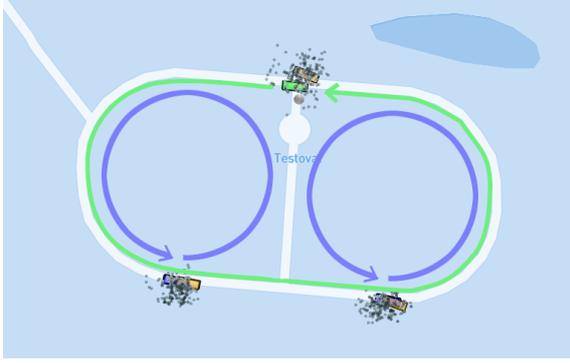
Figure 1: Simulation setup of the case study extracted from Streetscape.gl (Uber ATG and VIS.GL, 2020) visualization. Shown are the VuT in green and the two target vehicles in purple as well as their corresponding driving trajectories. Additionally, in orange are the position as given by the simulated GPS sensor. The point clouds represent position hypotheses generated by the particle filter.
