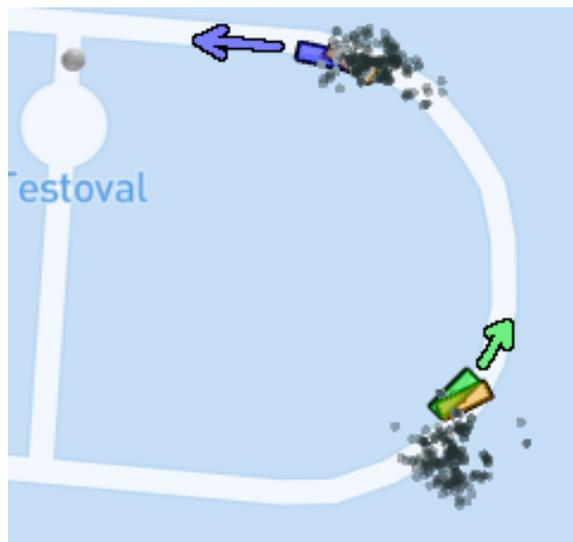
Figure 4: Vehicle configuration at  $t = 20$ s. Both vehicles are moving anti-clockwise as shown. At this time instance, the green VuT moves with 50km/h whereas the violet participant moves at 18km/h.
