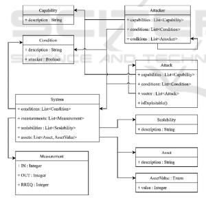
Figure 4: Data Model to store to link Security-relevant Information and the Specification.
