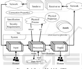
Figure 2: A System Model for CPS.
