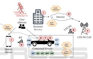
Figure 1: A prototypical Car Sharing Application.
