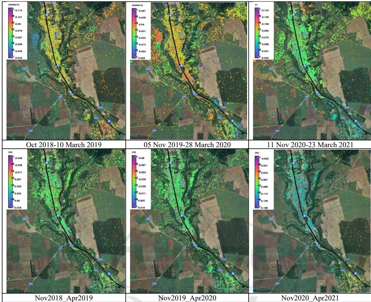
Figure 5: Subset of displacement maps created from SAR data satellite orbits 36 and 58 (black line is the monitored railway line).
