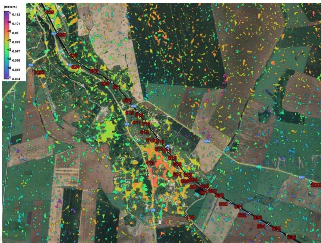
Figure 4: Subset of displacement map for the period Oct 2018-10 March 2019 and geodetic points from railway route.
