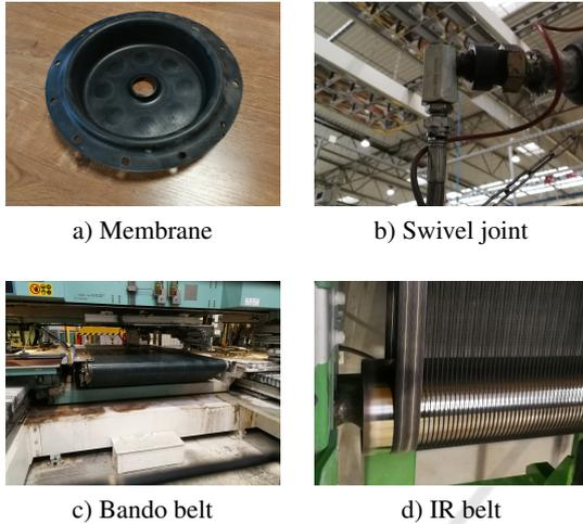
Figure 4: Industrial spare parts used as examples for maintenance cost optimisation.
