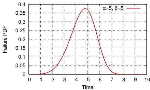
Figure 1: Probability density for the Weibull distribution with  $\alpha = 5$  and  $\beta = 5$ .
