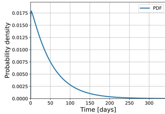
Figure 6: Membrane Weibull PDF for  $\alpha = 51.559$  and  $\beta = 1.021$ .
