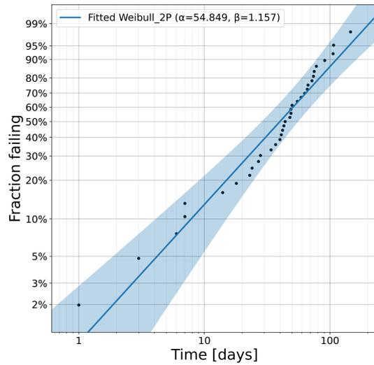
Figure 9: Bando belt Weibull probability plot determined by coordinate linearization and less square method.
