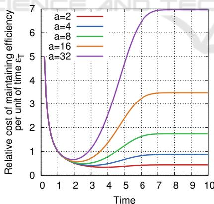
Figure 2: The functions of the relative cost of maintaining efficiency in the time unit  $\epsilon_T$  for example values of the  $a$  parameter and the Weibull distribution with the parameters  $\alpha = \beta = 5$ .
