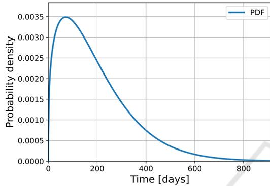
Figure 8: Swivel joint Weibull PDF for  $\alpha = 210.551$  and  $\beta = 1.317$ .
