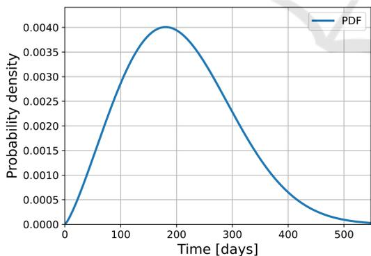
Figure 12: IR belt Weibull PDF for  $\alpha = 233.461$  and  $\beta = 2.264$ .
