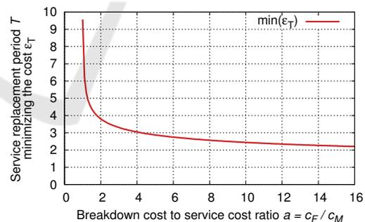
Figure 3: Values of  $T$  minimizing the relative cost of maintaining efficiency in the time unit  $\epsilon_T$  for the given values of the parameter  $a$ .
