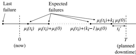
Figure 14: Expected failures in the case of not carry out preventive replacement of the element.
