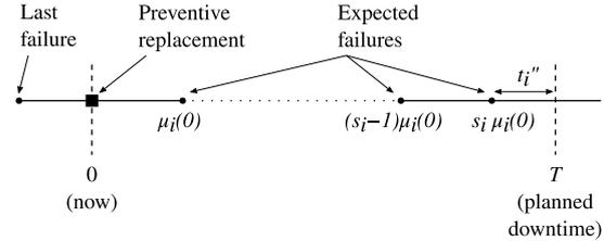
Figure 15: Expected failures in the event of a preventive replacement of an element.
