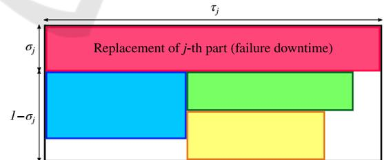
Figure 16: Optimum use of downtime for the preventive replacement of additional parts.
