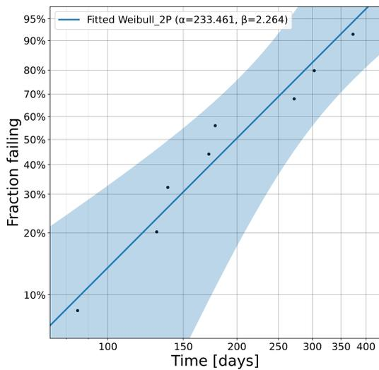
Figure 11: IR belt Weibull probability plot determined by coordinate linearization and less square method.
