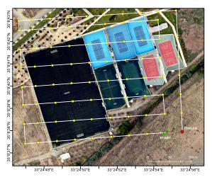
Figure 2: Flight plan of the surveyed area. The dots indicate the waypoints of the strips.
