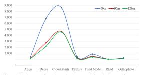
Figure 5: Processing time (sec) per altitude for each examined parameter.
