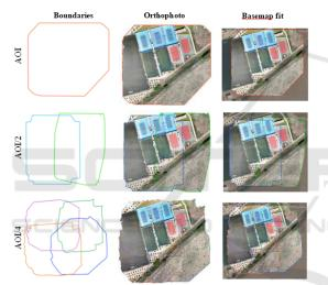
Figure 8: Resulted orthophotos for each flight with different AOI boundaries, compared to the respect scene of Google satellite basemap.
