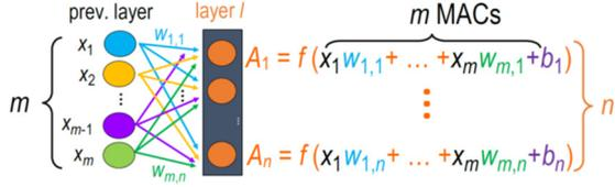
Figure 6: Computation and associated data in FC layer 1
