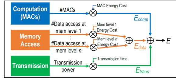
Figure 2: Energy consumption methodology of a computing unit<sup>1</sup>
