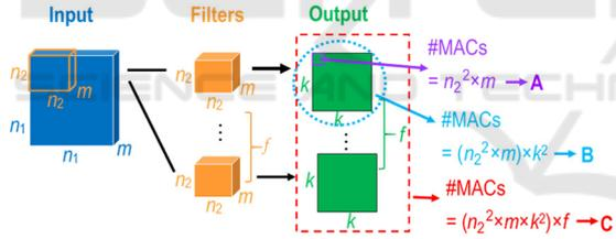
Figure 7: Computation and associated data in CONV layer.
