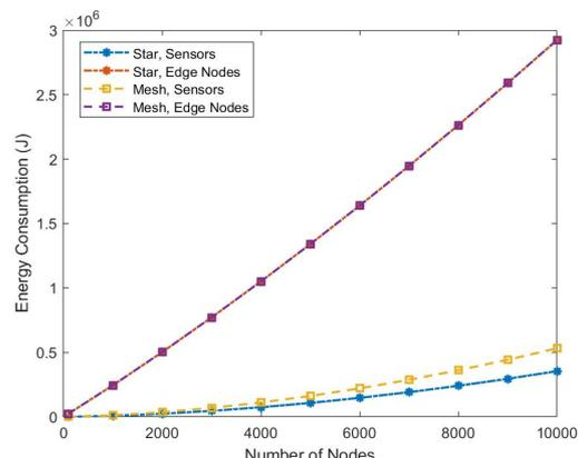
Figure 10: Energy consumption of sensors vs. distributed servers (edge nodes).
