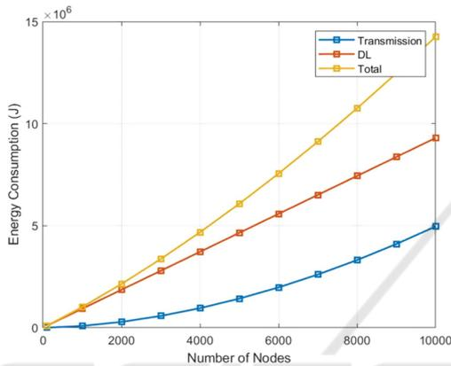
Figure 11: Energy consumption where bandwidth is 2MHz.
