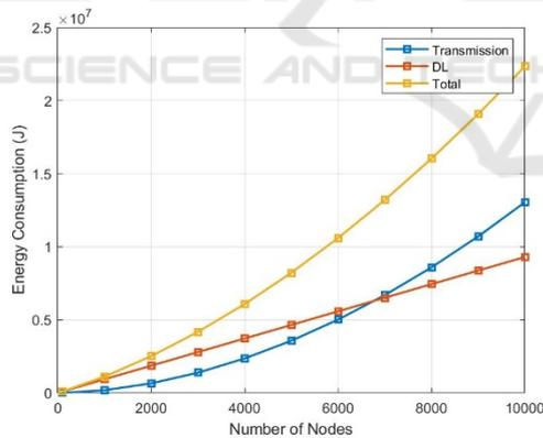
Figure 12: Energy consumption where bandwidth is 500kHz.
