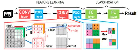
Figure 5: A Convolutional Neural Network (CNN)1
