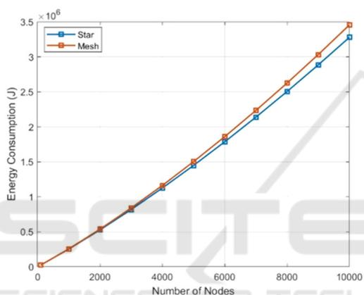
Figure 9: Energy consumption of star and mesh networks.
