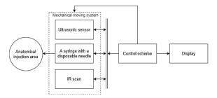
Figure 1: Generalized structure of the automatic drug injection system.
