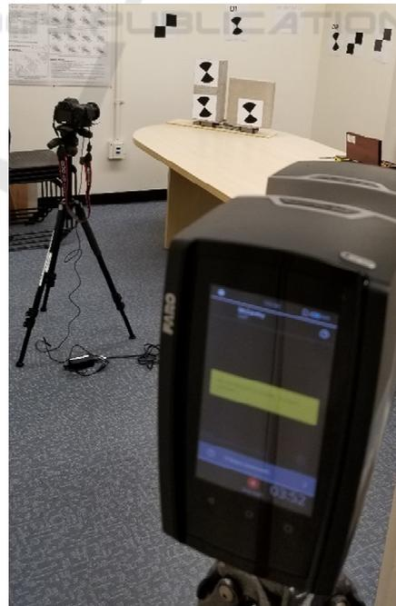
Figure 3: Terrestrial laser scanner used in the setup.
