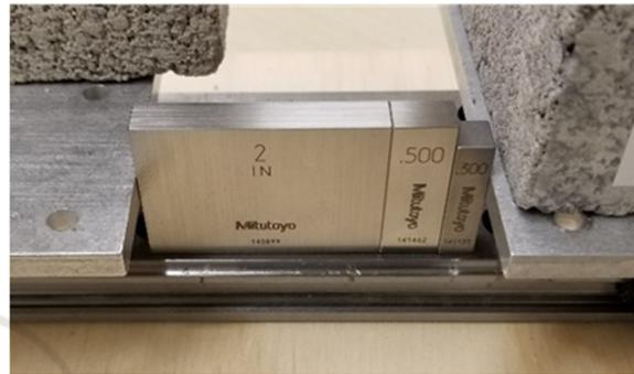
Figure 2: Displacement between carriages set by high-precision blocks.
