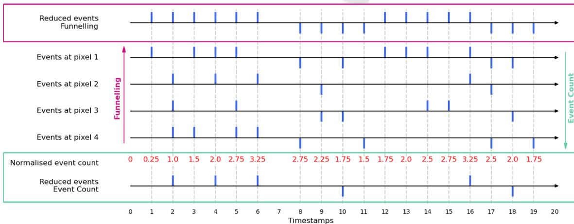
Figure 4: Schematic illustration for event funnelling and event counts methods. A sensor of size  $2 \times 2$  outputs negative and positive at each pixel across time, which are downsampled using Simple Event Funnelling (red frame on top) and Log-Luminance Event count (green frame at the bottom). In this example, the downscaling factor is set to 2.
