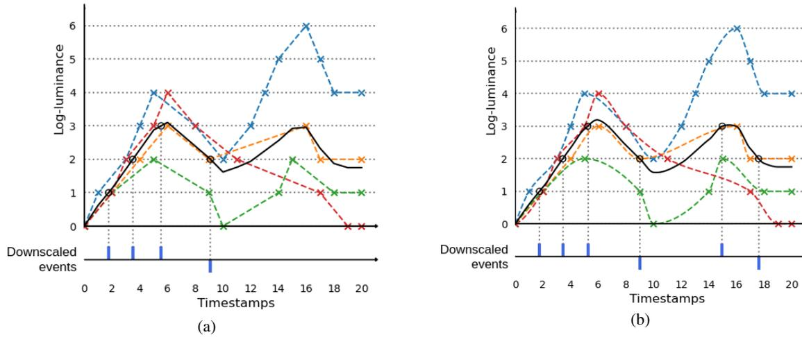
Figure 5: Schematic illustration for log-luminance reconstruction. A sensor of size  $2 \times 2$  outputs negative and positive at each pixel across time, which are downsampled using log-luminance reconstruction with linear (a) and cubic (b) interpolation. In this example, the downscaling factor is set to 2.
