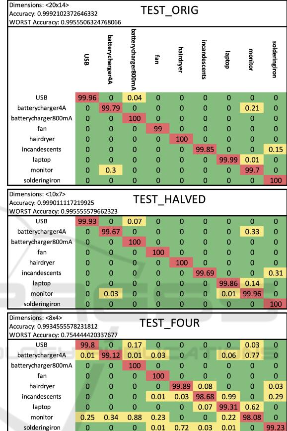
Figure 12: Confusion matrix (average of 100 runs) of the CNN classification results. A common USB class was used for the three USB adapters, and the incandescent light bulb and the infrared lamp were merged to one class (incandescents). 150 samples from each class were used for training the model, 100 were used for testing.
