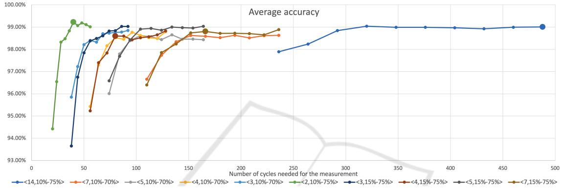
Figure 8: Average simulation results plotted for each cutoff ratio set. The bigger markers show the measurement profiles chosen. The horizontal axis shows the number of cycles each measurement would take assuming  $d = 16$ .
