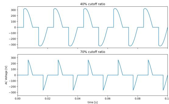
Figure 1: Voltage cutoff method with different cutoff ratios. collecting data about the devices' characteristic response.
