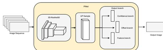
Figure 4: 3D ResNet is integrated with PINet for feature extraction.
