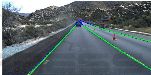
(a) The result of lane marking detection.
