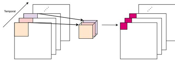
Figure 2: The 3D ConvNets (or 3D CNN) used to extract the time and space information from an image sequence.
