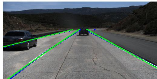
Figure 12: The lane detection result from PINet 3D-ResNet50-2P1D.
