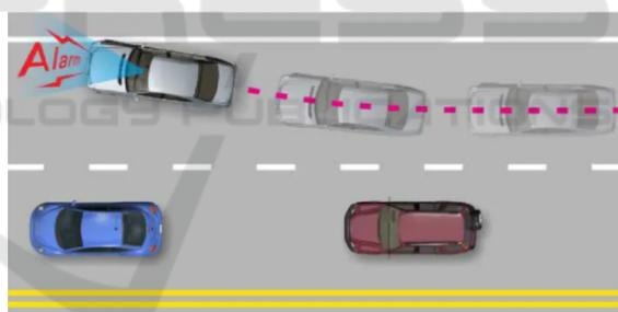
Figure 1: An illustration of the lane departure warning for driver assistance.
