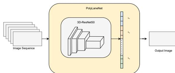
Figure 3: PolyLaneNet is improved with 3D ResNet by incorporating the temporal information.
