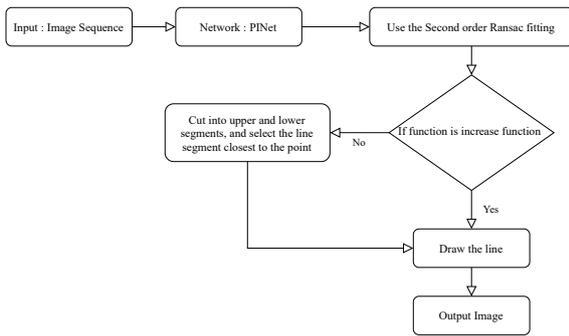
Figure 5: The system flowchart of our proposed lane marking detection algorithm.
