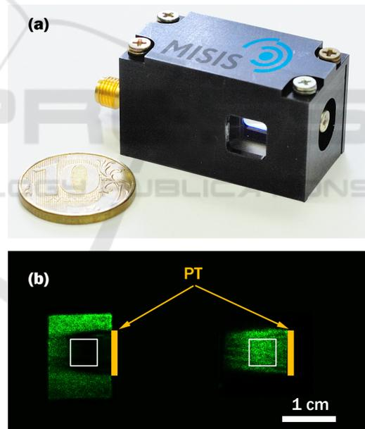
Figure 1: Noncollinear paratellurite AOTF: (a) real-size photograph; (b) acoustic field visualization: left — 0<sup>th</sup> order; right — 1<sup>st</sup> order; white rectangle — optical aperture; yellow rectangle — piezotransducer (PT).
