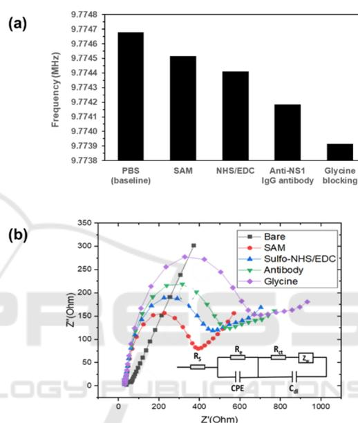
Figure 4: Change of frequency (a) and Nyquist impedance diagrams (b) of a surface functionalized IEQCM, layer-by-layer: bare electrode, SAM, NHS/EDC, dengue anti-NS1 capture antibody, and blocking agent glycine. Surface modification experiments were performed with  $n = 1$ .
