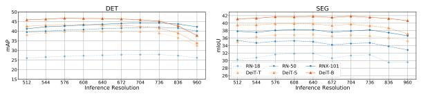
Figure 3: Comparison of VTs and their CNN counterparts at inference resolutions higher than training resolution (512 × 512).
