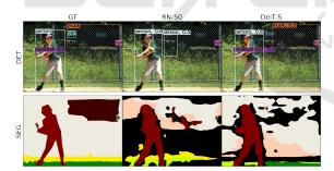
Figure 8: Qualitative comparison of DeiT-S and RN-50 predictions under targeted attack with 'person' and 'car' classes swapped. RN-50 predicts 'person' class for 'car' region in detection and segmentation.
