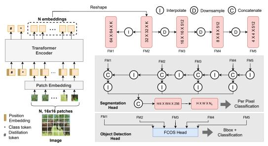
Figure 1: Architecture for object detection and semantic segmentation with VT backbone.
