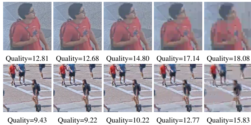
Figure 5: Figure shows image quality for frame of video compressed using different compression parameter. Each row shows patch from frame of a video. Each column shows the images compressed with same compression parameter. CRF-23, CRF-29, CRF-35, CRF-41, CRF-47 are compression parameters for each column respectively.
