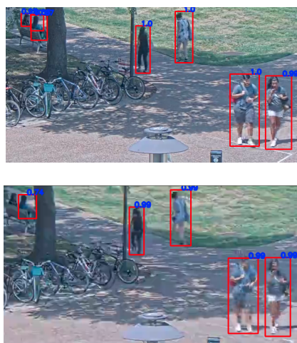
Figure 2: Figure shows result of Faster RCNN (Ren et al. , 2015) object detection model on a low compressed frame (top) and highly compressed frame (bottom).
