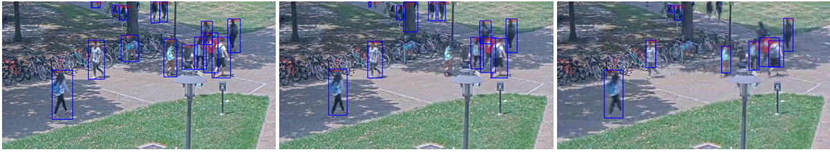
Figure 1: Figure shows object detection results on a sample frame from a video. (Left) Frame is from a video that is uncompressed. All the objects in the images are detected. (Middle) There are 4 objects that are not detected after applying low compression. (Right) The number of objects that are not detected has increased with increased compression.
