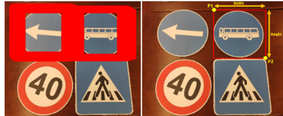
Figure 6: All detections with confidence scores over 40% (Left). Detection with the highest confidence score (Right).
