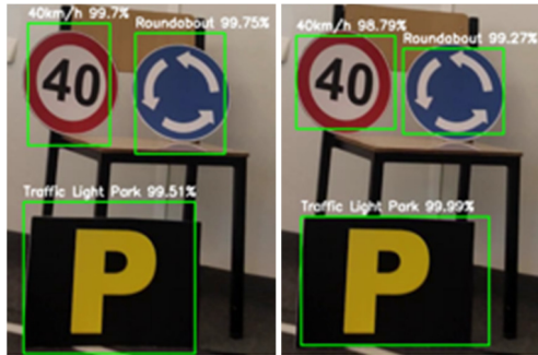
Figure 16: Detection from the YOLOV3 (left) and YOLOV3_tiny (right).
