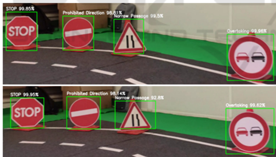
Figure 17: Bounding Boxes from the YOLOV3 (top) and YOLOV3_tiny (bottom).
