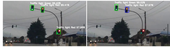
Figure 22: Traffic Light detection from the YOLOV3 (left) and YOLOV3_tiny (right).
