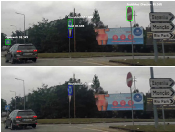
Figure 20: Detection with rain from the YOLOV3 (top) and YOLOV3_tiny (bottom).
