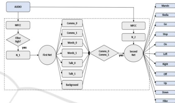
Figure 3: Vocal command recognition system diagram.
