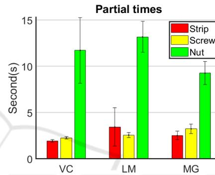
Figure 4: Partial time (in seconds, averaged across participants, with standard error of the mean) to put in the correct position the three considered objects. VC: Vive Controllers, LM: Leap Motion, MG: Manus Gloves.
