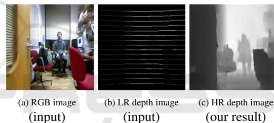
Figure 1: High resolution depth image generated from low-resolution depth image of LiDAR by using our proposed method. The low-resolution depth image is considered as defect image with holes and image inpainting is conducted for obtaining high resolution depth image with the proposed method.
