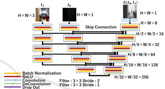
Figure 4: Generator of Proposed method 2.
