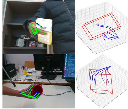
Figure 9: 3D hand and object pose on HO3D validation samples.
