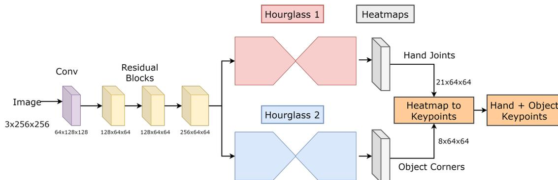
Figure 3: The architecture of 2D hand pose and 2D object corner regression using heatmaps.
