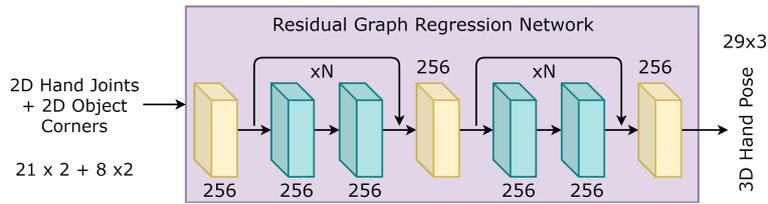
Figure 4: The architecture of residual graph regression network for 3D pose regression.
