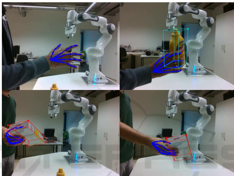
Figure 12: Hand and object pose estimation in human-robot interaction environment.
