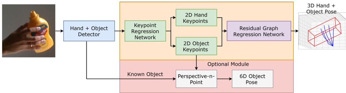
Figure 1: The overview of complete pipeline. The input is an RGB image and output is the 2D hand pose, 2D object corners, 3D object corners, 3D hand pose and an optional module to get 6D object pose using perspective-n-point algorithm.
