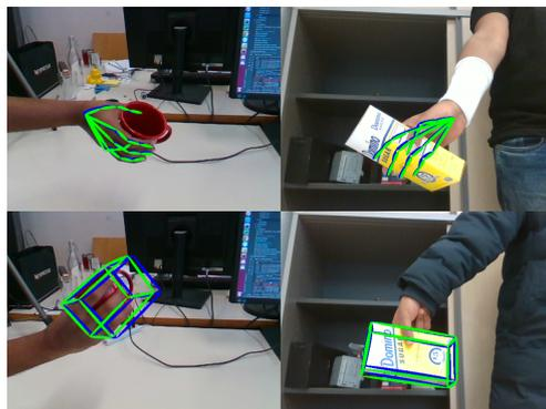
Figure 7: The 2D hand pose and object pose outputs. The green lines represent groundtruth and the blue lines indicate predicted keypoints.
