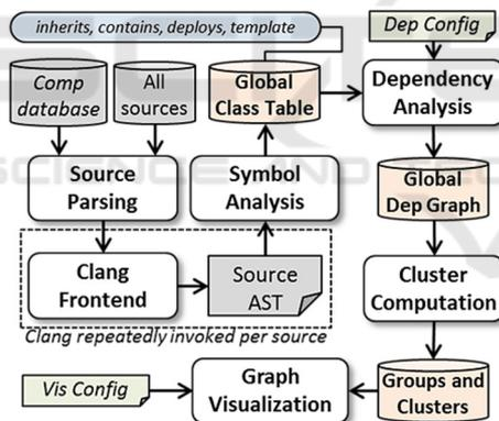
Figure 2: Overview of the miner software architecture.
