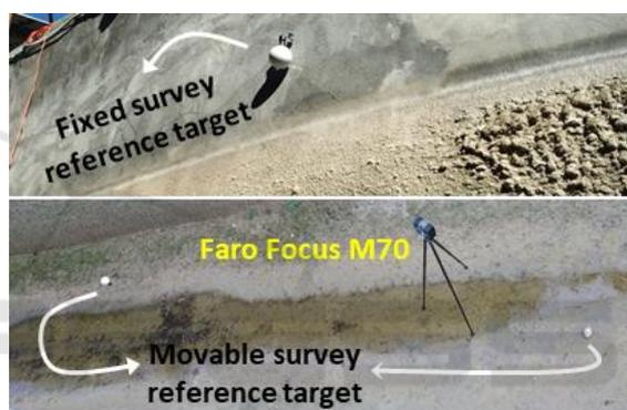
Figure 8: Terrestrial laser scanning of tufa tunnel.
