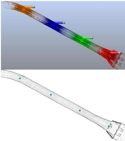
Figure 17: Point cloud of tufa tunnel section with four scan location.
