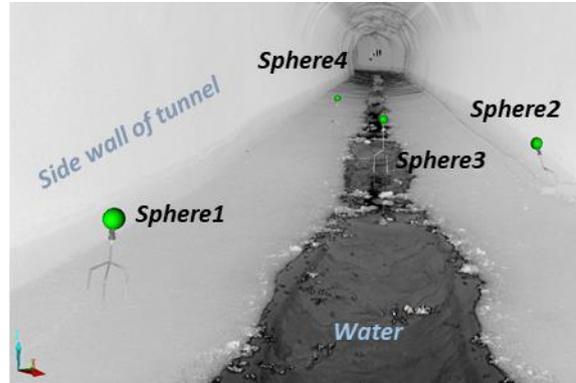
Figure 12: Recognized spheres at eighth scan station.
