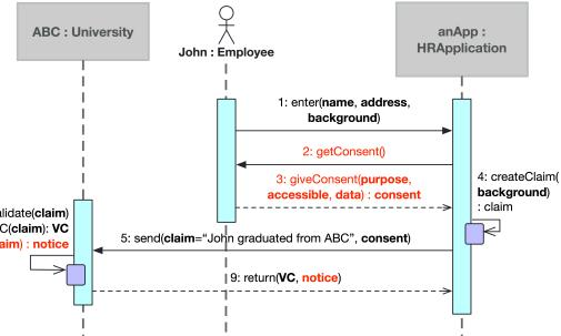
Figure 4: A use case for the HR application's service authentication scenario.
